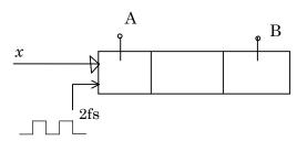
The frequency of signal *x* is fs and the shift register is clocked at the positive edge of 2fs. The time offset between A and B is
