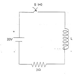
For the circuit shown in the figure, the switch is closed at t=0. After some time when the current in the inductor was 6A, the rate of change of current through the inductor was 4A/sec. The value of the inductor is
