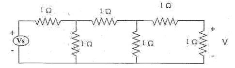
The Voltage across last resistor is V. All resistors are unity. Then Vs is given by
