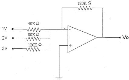
In the circuit shown in the above figure, the value of output V<sub>0</sub> is
