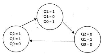
It is designed using D F/Fs and combinational logic blocks  $L_1$ ,  $L_2$  &  $L_3$  and is initialized at  $(Q_2=1, Q_1=0, Q_0=1)$
