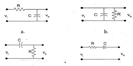
(17) For a parallel RC circuit as shown in figure, R = 20  $\Omega$  & C = 0.9 pF , which is to be matched to  $50\Omega$  over a bandwidth,
