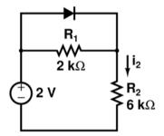
The magnitude of the current i<sub>2</sub> (in mA) is equal to \_\_\_\_\_
