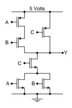
(A)  $Y = \overline{A} \overline{B} + \overline{C}$
