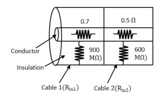
$$\begin{split} \left(R_{eq}\right)_{conductor} &= 0.7 + 0.5 = 1.2\Omega \\ \left(R_{eq}\right)_{in} &= \frac{1}{\left(R_{eq}\right)_{in}} = \frac{1}{\left(R_{in}\right)_{1}} + \frac{1}{\left(R_{in}\right)_{2}} = \frac{1}{900 \times 10^{6}} + \frac{1}{600 \times 10^{6}} \\ \left(R_{eq}\right)_{in} &= 360 \times 10^{6}\Omega \\ \hline \left(R_{eq}\right)_{in} &= \frac{360 \times 10^{6}}{1.2} = 300 \times 10^{6}. \end{split}$$
