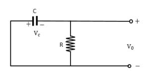
$$\begin{split} V_c(f) &= V_c \left(\frac{T}{2}\right) e^{-t(t-T/2)\tau} \\ & \therefore V_c(t) = V_{c \text{ max}} e^{-(t-T/2)\tau} \\ & \text{ at } t = T, V_c = V_{c \text{ min}} \\ & \Rightarrow V_{c \text{ min}} = V_{c \text{max}} e^{-T/2\tau} \\ & \text{As } V_{c \text{ max}} - V_{c \text{ max}} = 1.2 \\ & \text{ [From ($\alpha$)]} \end{split}$$
