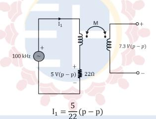
$$V_0 = j\omega MI_1 = 7.3 = (2\pi \times 10 \times 10^3) \times M \times (\frac{5}{22})$$
