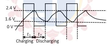
$$V_c(t) = V_{c \, final} + [V_{initial} - V_{c' final}]e^{-t/RC}$$
